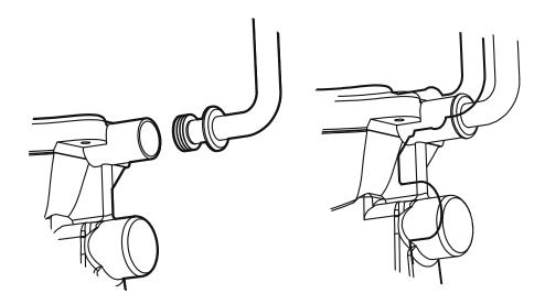
2.Insert the flush pipe and flush cone into the inlet hole on the pan. Ensure the pipe is fitted securely into the pan. Use a small dab of silicone to hold the metal cover in place.
