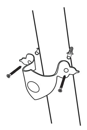
3. Use the pipe bracket to fix the pipe to the wall. Mount this bracket about halfway up the flush pipe.
