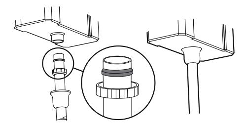
1.Insert the flush pipe into the bottom of the cistern and tighten the compression fitting. To ensure a good seal use PTFE tape, around the thread. Move the cover over the base of the flush valve and move the O-ring so it stays in position.
